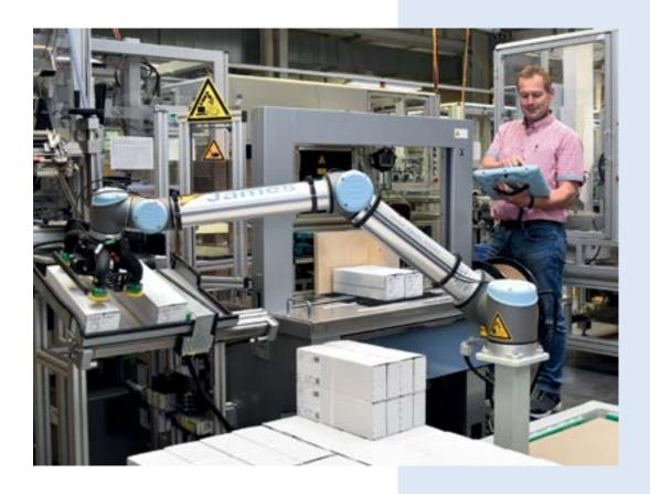
Palletizing procedures are monotonous, tedious, and time-consuming. This is one part of the value chain that employees least look forward to, making it ideal for automation. Cobots with an increased maximum payload of 16 kg boost palletizing performance by eliminating the need to handle heavy bulk products such as packaged animal feed and potting soil manually.
